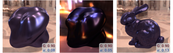
Fig. 15. Example of BRDF editing using our predictor under a different illumination (center) and geometry (right). We set the target glossiness to 0.9. Our predictor takes into account changes in illumination and geometry and updates \alpha accordingly.
